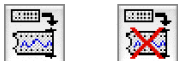
Figure 2-9 Record/Monitor button: left, data displayed and recorded; right, data displayed but not recorded.
