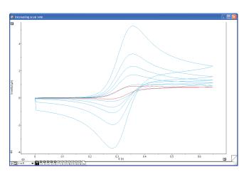
Cyclic voltammetry of a ferrocene derivative, at increasing scan rates, using EChem software
